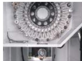
Equipped with the newly developed direct ATC type 30-tool magazine. Supports maximum tool length of 250 mm, maximum tool diameter of 125 mm, and maximum tool weight of 4 kg, enabling a variety of machining, including long workpieces.
