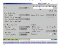
The current power consumption is shown on the screen, along with the maximum power consumption value, the power consumption record, the cumulative power consumption, and the power regeneration (generation) status. Data can be output, too.
